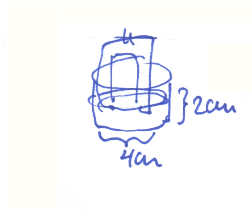
Figure 20: Arduino electrode and water in a glass, See section 3.84
