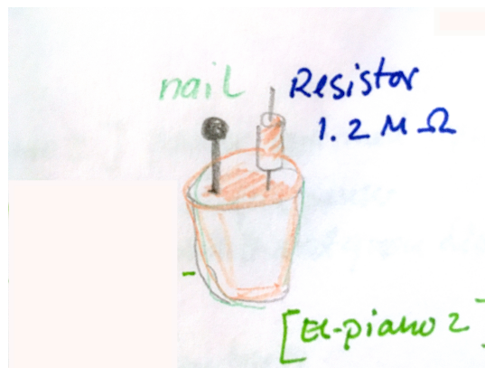
Figure 7: Pot with soil and grounding nail/resistor. See section 3.21
